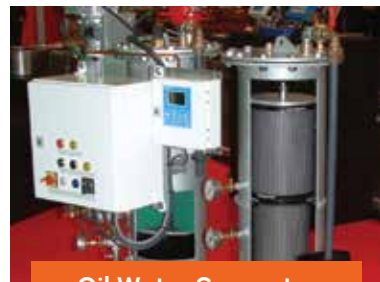
Oil Water Separator
